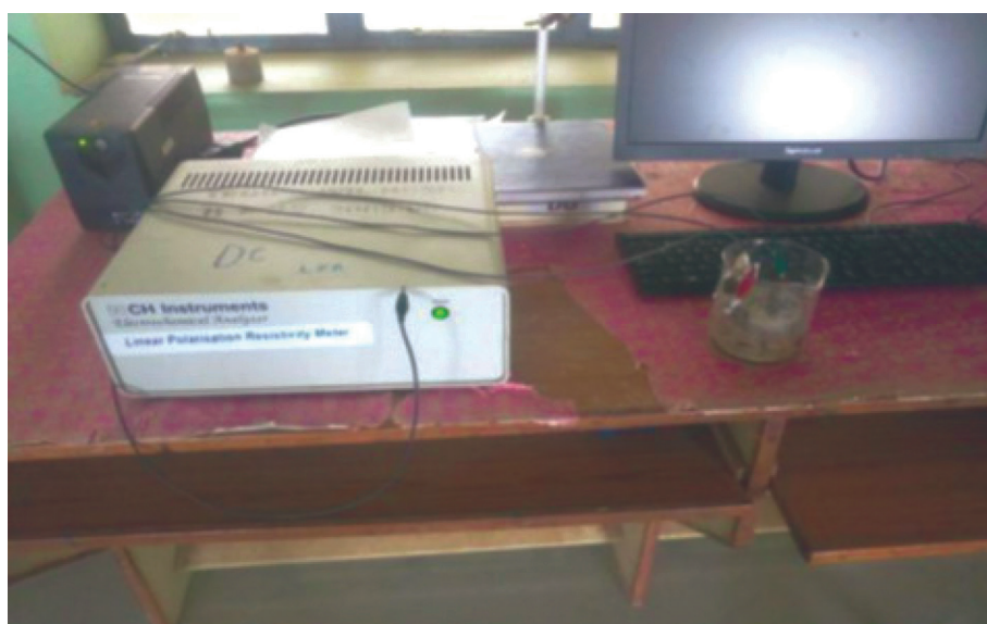
Fig. 6. Test set up for corrosion rate.
