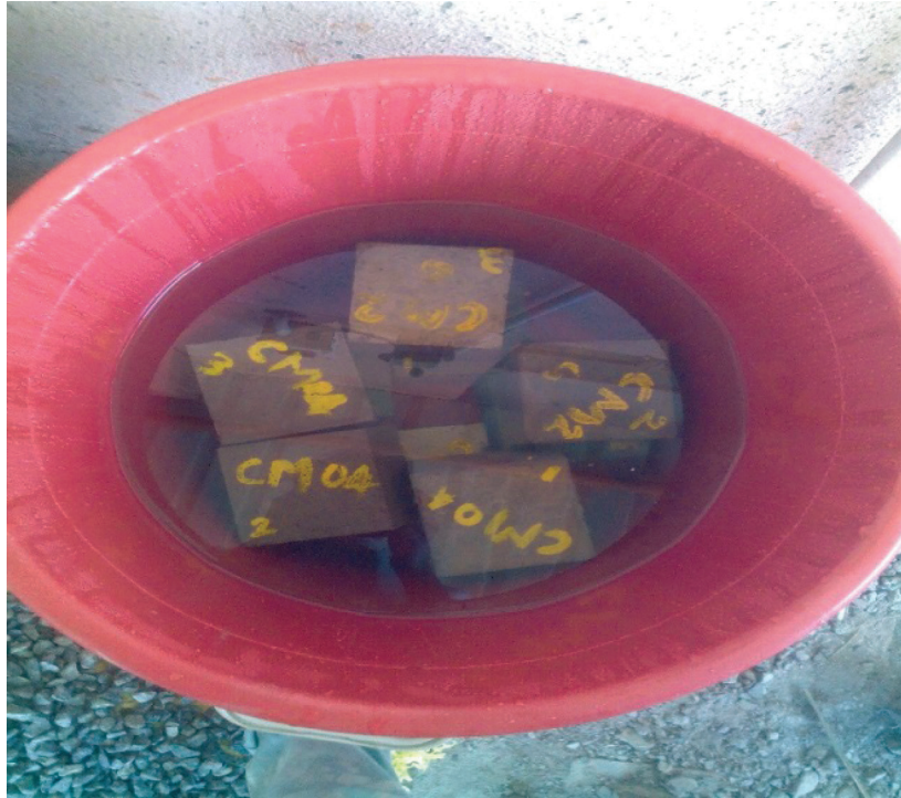
Fig. 4. Specimens soaked in acid solution for acid resistance test.
