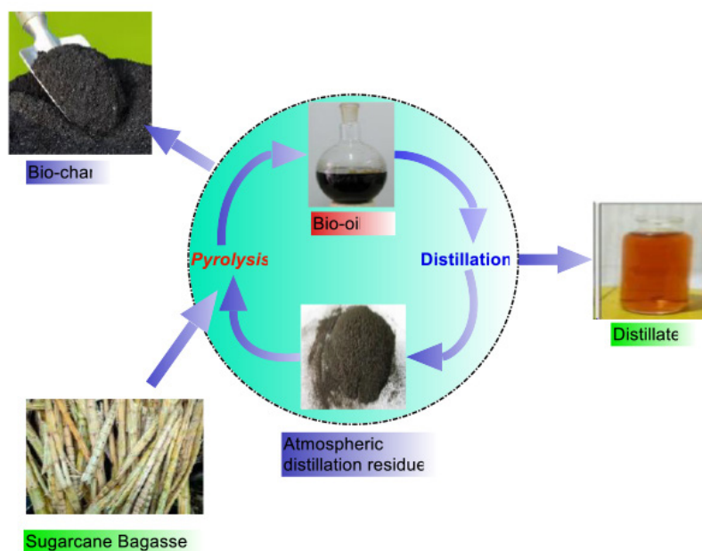
Fig. 4. Production of BO from SCB by fast pyrolysis [26]. Adapted from Zhang et al. (2013).
