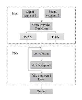
Fig. 9. The flow chart of the proposed approach based on CNN.
