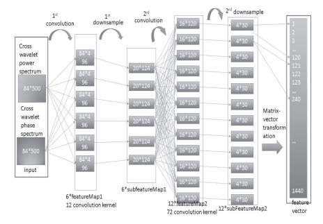
Fig. 8. The architecture of the proposed CNN model.
