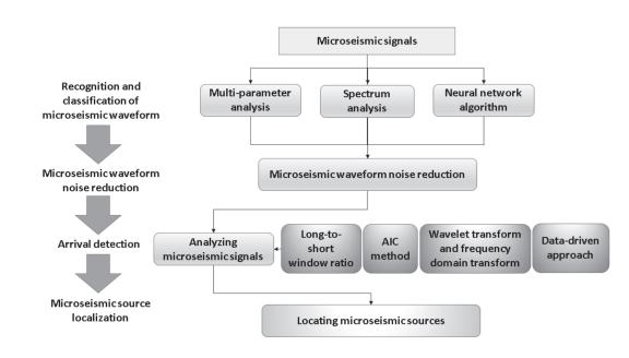
Fig. 6. Processing process of a microseismic signal.
