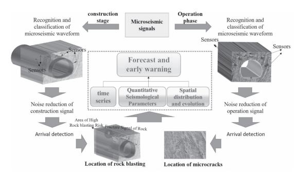
Fig. 10. Forecast and early warning process based on microseismic monitoring.
