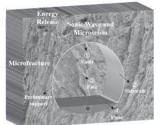
Fig. 3. Process of microfractures due to microseismics.
