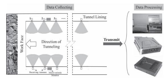
Fig. 2. Microseismic monitoring in tunnels.
