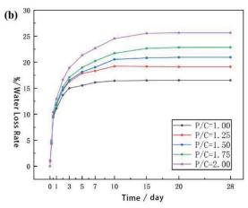
Fig. 1. a) Effect of 0-3 days P/C ratio on the water loss rate of the solid; b) Effect of 0-28 days P/C ratio on the water loss rate of the solid.
