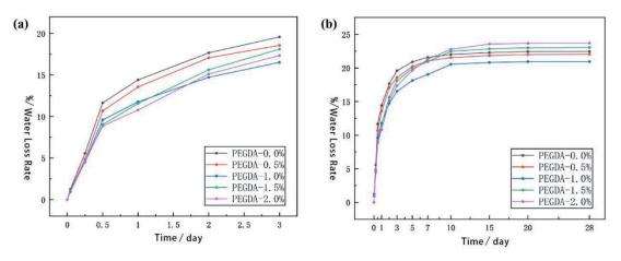
Fig. 3. a) Effect of 0-3 days cross-linking agent on water loss from the solid; (b Effect of 0-28 days cross-linking agent on water loss from the solid.
