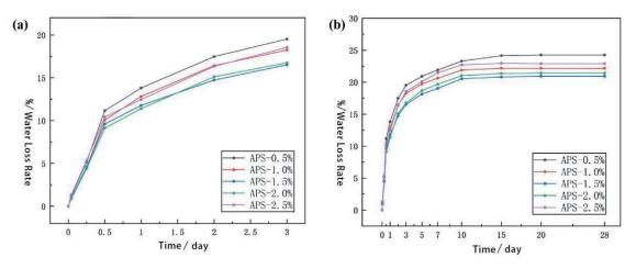
Fig. 2. a) Effect of 0-3 days initiator on water loss from solid; b) Effect of 0-28 days initiator on water loss from solid.
