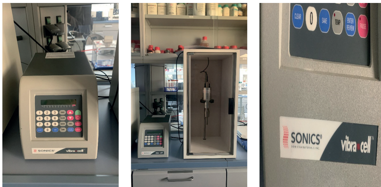
Fig. 1. The Vibra Cell Ultrasonic (CV334) sonication machine use in this study.
