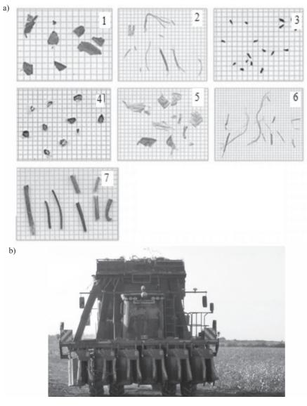
Fig. 1. Classification of machine and hand picked cotton pollution a) 1 - leaf, 2 - stem, 3 - funiculi 4 - seed coat, 5 - shale, 6 - grass, 7 - steck; John Deere is a cotton picker b).
