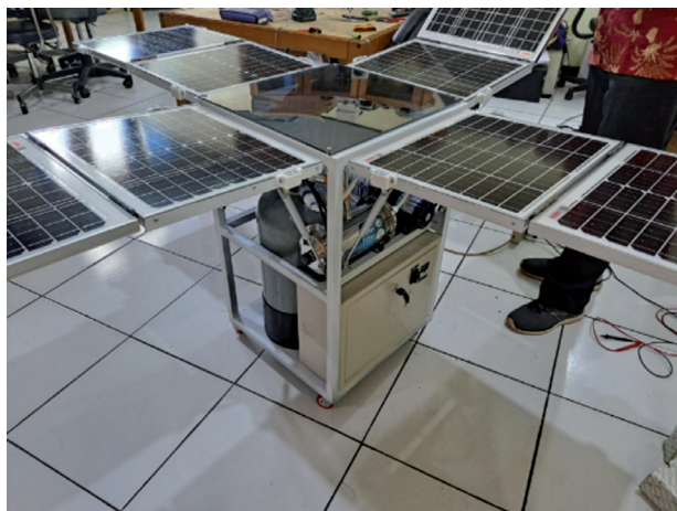
Fig. 1. Portable South Kalimantan peat water treatment solar-powered
