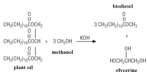
Fig. 1. Reaction for biodiesel oil production
