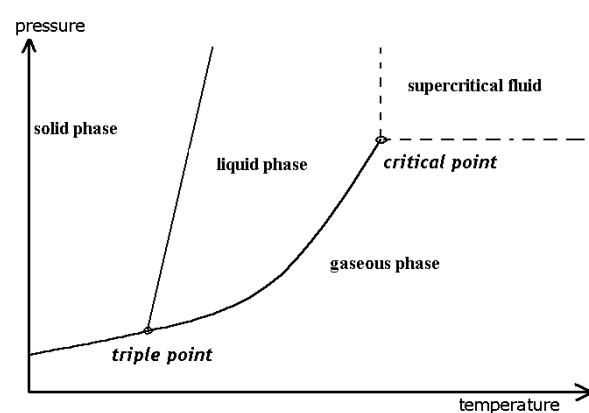
Fig. 2 Phase diagram showing supercritical fluid region.
