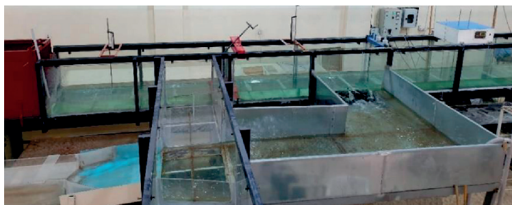
Fig. 1. Open channel flume used for the present study.
