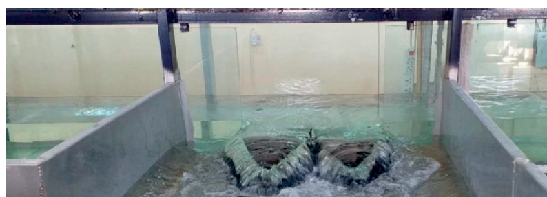
Fig. 7. The triangular labyrinth side weir experimental test.
