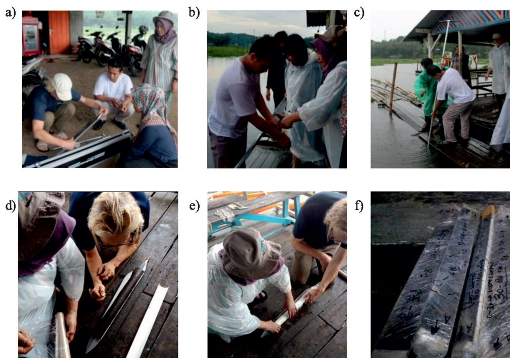
Fig. 2. Series of Sediment Coring Activities in the Upper Tuntang River (Rawapening Lake Outlet), Corer Installation a), Seeting Corer Before Use b), Sediment Coring c), Sediment Results Coring d), Sediment Wrapping Using Plastic Pipes e), and Wrapped Sediments for Further Analysis f).
